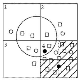
Figure 3 - 'Clumping' with dynamic load balancing
