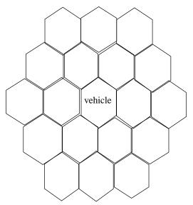
is associated with a multicast group. In the figure above we associate a vehicle with 19 hexagons that represent its AOI. Hence, it is also a member of 19 network multicast groups. The entity's host listens to all 19 groups but, with two exceptions, it sends PDUs only to the one associated with the cell in which it is located.
