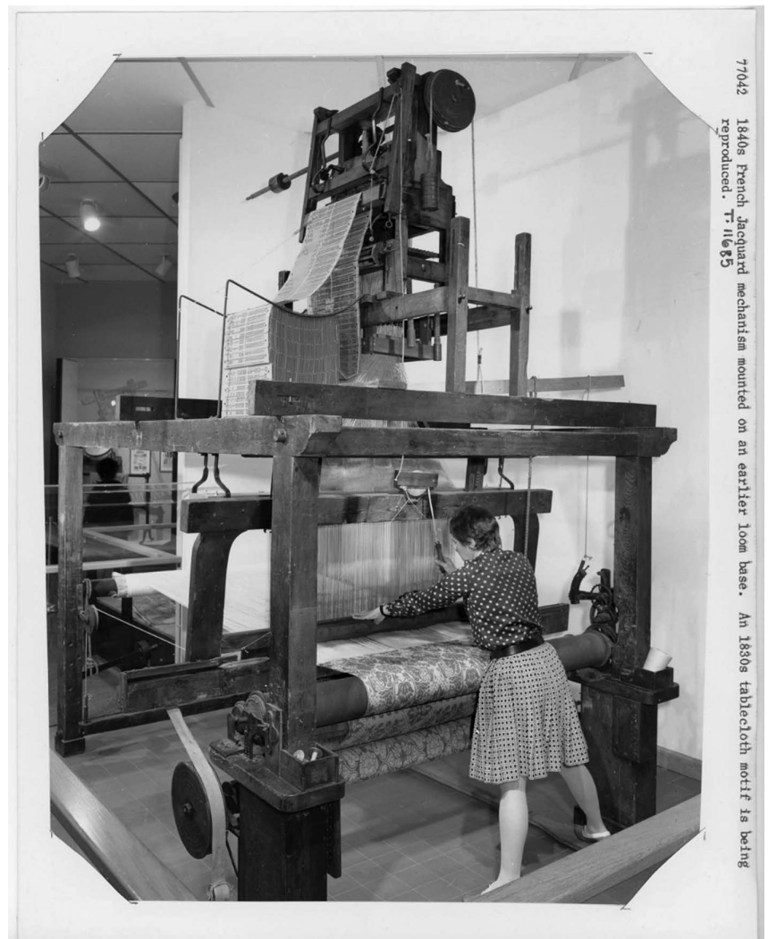
FIGURE 1. The Jacquard loom system. Jacquard's mechanical loom was integrated with a punched card control mechanism. The card system (at the top of the picture) encodes the patterns that guide the loom's weaving operations and outputs (shown at the bottom of the picture as a damask cloth), demonstrating an early example of programmable automation. 9
