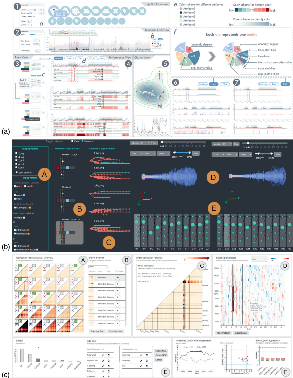
FIGURE 3. Promising visualization systems for DTs. (a) CloudDet: anomaly detection in cloud computing systems, 16 (b) a system for analyzing high-performance computing aircraft engine simulations. 17 (c) Irvine: a manufacturing system that analyzes correlation patterns of automotive electrical engines. 18
