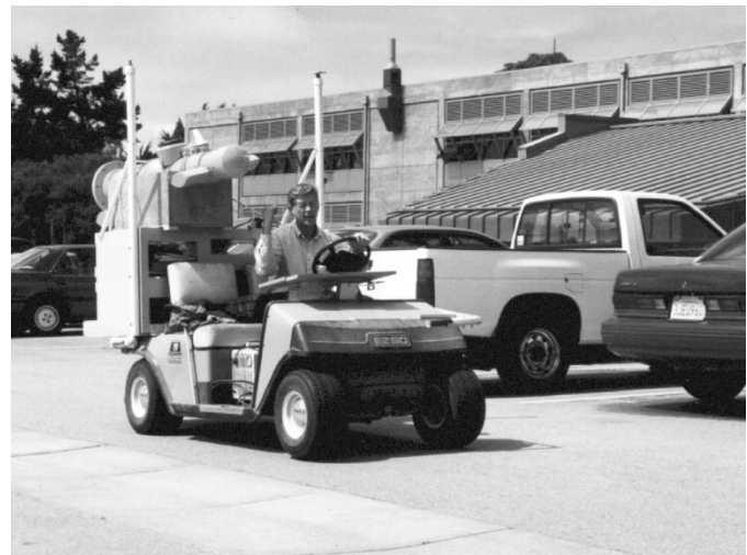
Fig. 12. The towfish mounted on a golf cart during parking lot testing.
