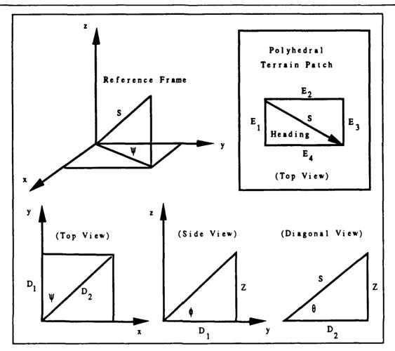
Figure 3.7 Heading Inclination Angle
