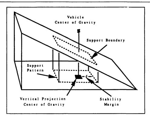
Figure 3.11 Three-dimensional Stability Model
