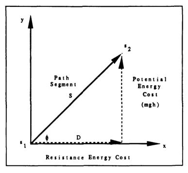
Figure 3.3 Components of Energy Cost
