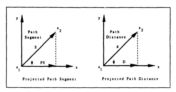
Figure 3.2 Single Path Segment and Projection
