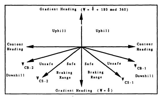
Figure 3.14 Critical Braking and Stability Headings
