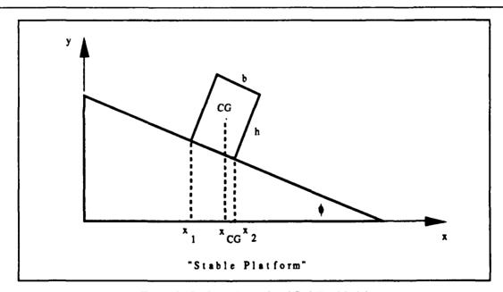
Figure 3.10 Two-dimensional Stability Model
