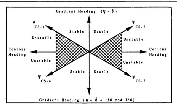
Figure 3.12 Critical Stability Headings
