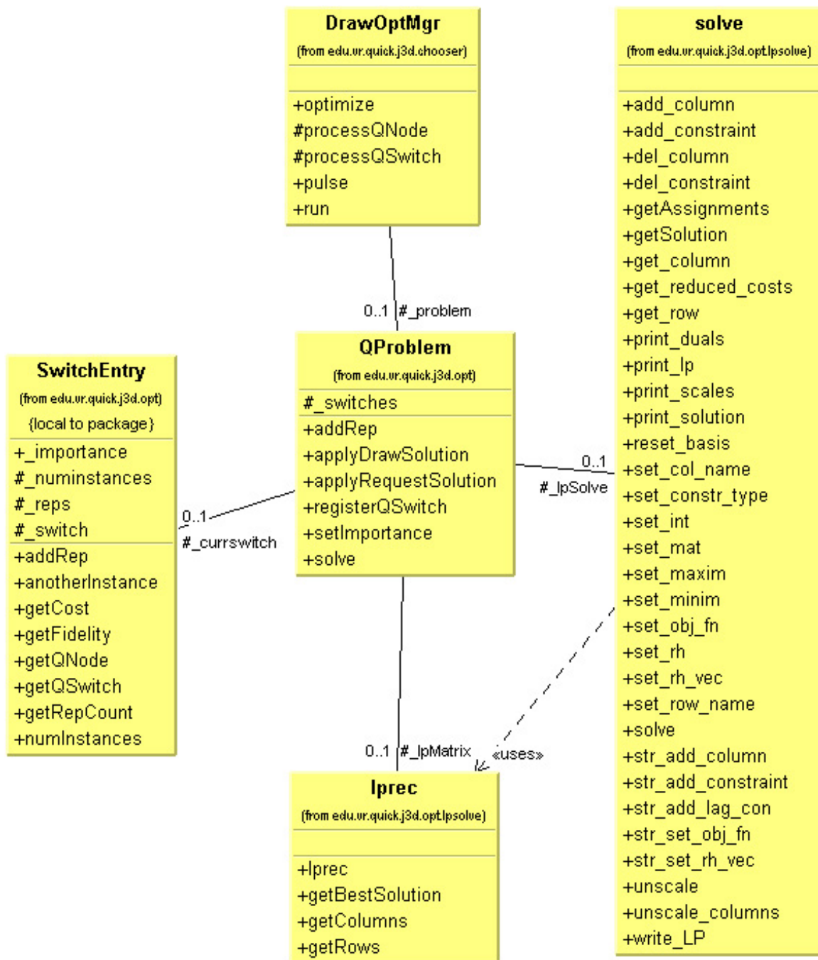
Figure 30. Class hierarchy diagrams for the edu.vr.quick.j3d.opt and ...opt.lpsolve packages.
