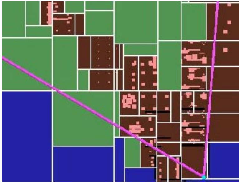
Figure 4. Dynamic visibility with the largest-occluder algorithm [Coorg and Teller, 1996].
